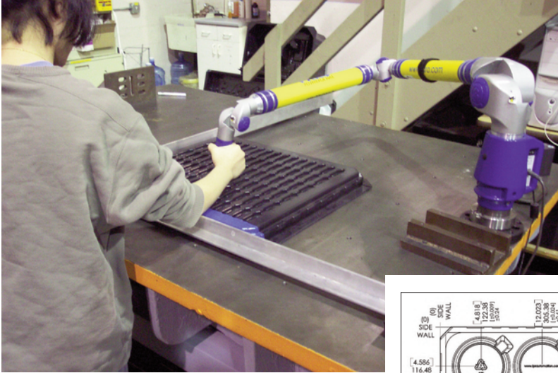
Measuring pocket to pocket repeatability with the faro arm
